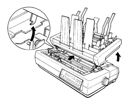
2. Replace the paper eject guide by fitting its notches onto the red pins inside the printer at each side, then tilting the paper eject guide back slightly.
